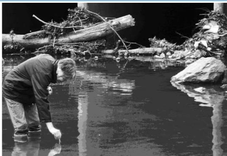
Figure 5. Volunteer Monitor Measuring Bacteria in a Local Stream. Save Our Saugahatchee citizen monitor testing local stream for E. coli (left), and results of incubated sample (right) showing extensive E. coli contamination.
