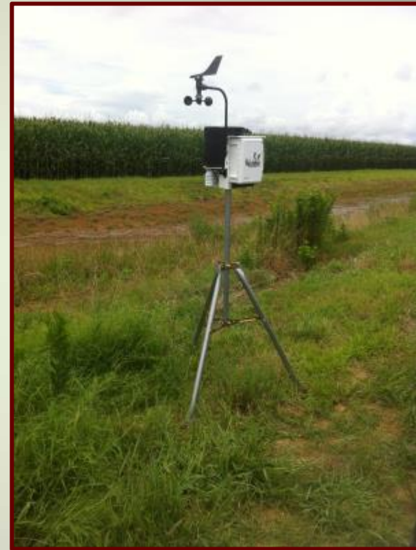
WatchDog 2900 ET weather station installed at the watershed
