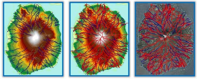
■ FAST quickly enabled an understanding of hydrologic drainage basins, then used to guide more detailed 1D modeling
