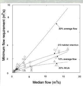
Trend lines of relationships between median flow and minimum flow requirements assessed using 10 % average flow, 30% average flow, minimum of 20% food-producing WUA, and retention of two-thirds of the food-producing habitat at median flow. Minimum flow requirements based on minimum habitat are shown as triangles, those based on habitat retention are shown as circles. Minimum flow requirements based on 10 and 30% average flow were close to the fitted lines and are not shown for clarity.
