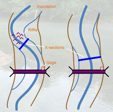
"Control" is the channel feature that determines water-surface elevation for a given flow rate
