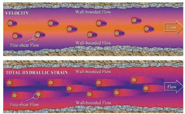
$$S_1 = \sum \left| \frac{\partial u_i}{\partial x_j} \right| = \left| \frac{\partial u}{\partial x} \right| + \left| \frac{\partial u}{\partial y} \right| + \left| \frac{\partial u}{\partial z} \right| + \left| \frac{\partial v}{\partial x} \right| + \left| \frac{\partial v}{\partial y} \right| + \left| \frac{\partial v}{\partial z} \right| + \left| \frac{\partial w}{\partial x} \right| + \left| \frac{\partial w}{\partial y} \right| + \left| \frac{\partial w}{\partial z} \right|$$
