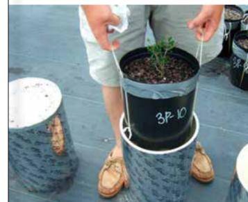
**LOSING GAS** A researcher lowers a 3-gallon dwarf yaupon holly into a flux chamber to measure the volume of greenhouse gas the plant is emitting. The study compared the gas emissions from four commonly used container sizes.
